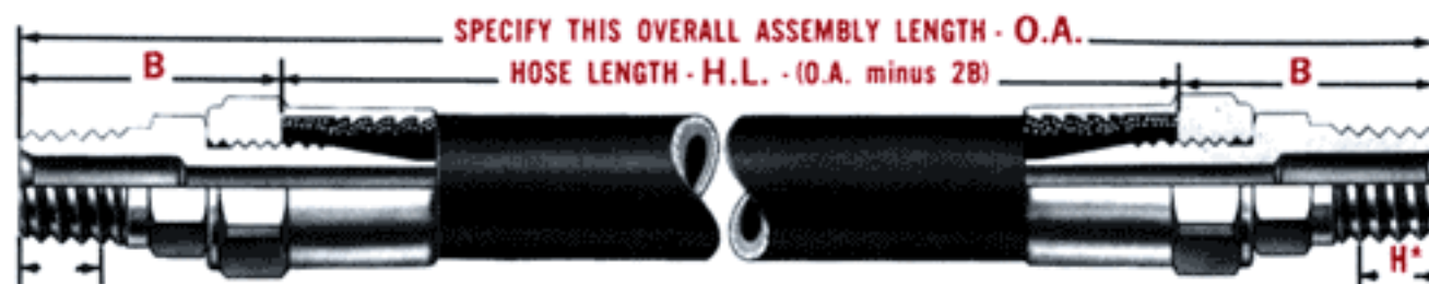
SHOWN ABOVE - AL and SAL ASSEMBLIES THROUGH \frac{1}{8} " I.D. HOSE SIZE (BRASS FITTINGS)
